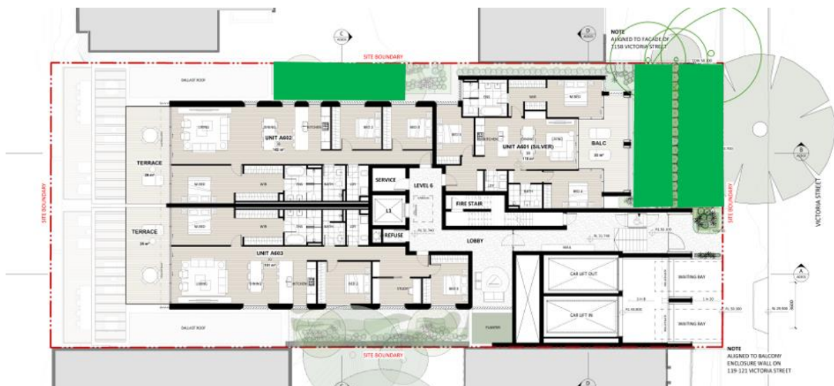
Figure 35: Excerpt of proposed deep soil areas to the front (east) and side (north) boundaries (highlighted in green)
